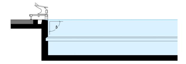
**PART 2, 16.2.5.2** - Rest ledges along the pool walls are permitted; they must be not less than 1.2m below the water surface and may be 0.1m to 0.15m wide. Both internal and external ledges are acceptable, however internal ledges are preferred.
