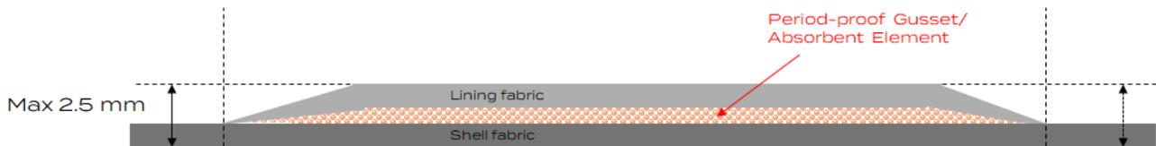
**B. Construction of the absorbent element/period-proof gusset**
